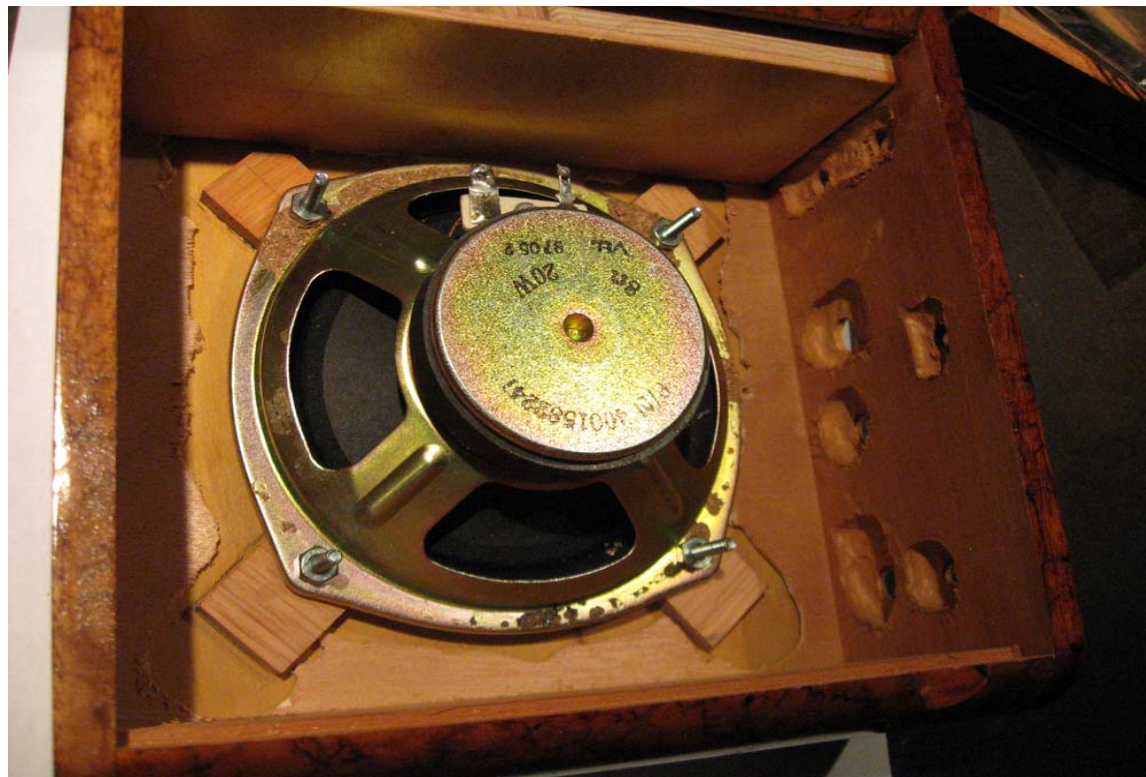
Face on Box & Control Cavities Created
